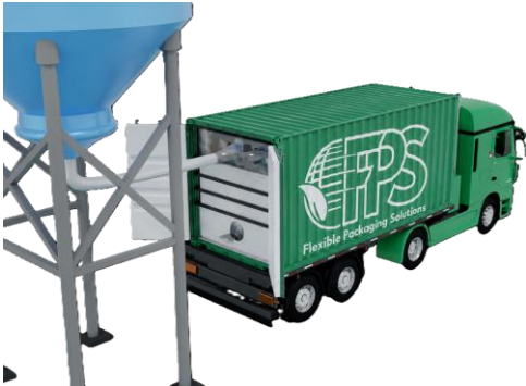
Silo to Container Liner direct transfer with Pneumatic Equipment
