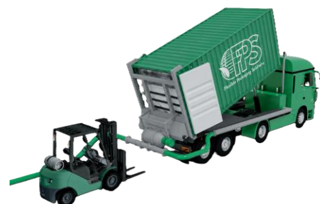
Container Liner discharge by Gravity + Pneumatics from Self-Discharge Truck with Hydraulic Tilting Chassis + Built-in Rotary Valve and Blower package
