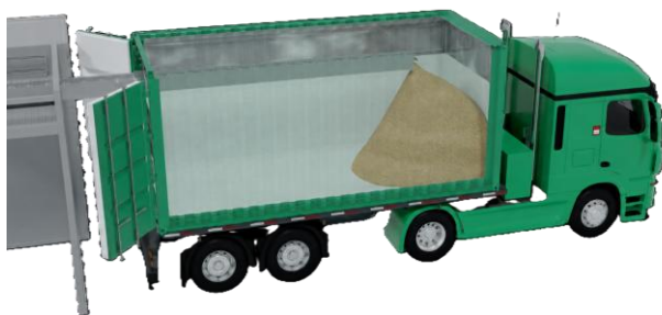
Silo to Container Liner direct transfer with SCREW CONVEYOR Equipment
