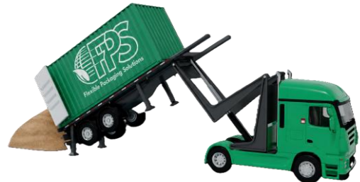
Container Liner discharge by gravity with 5th Wheel Hoist Tilt Tractor Truck
